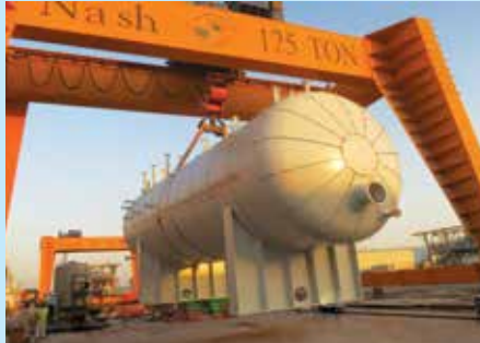
BUFFER DEGASSER VESSEL
